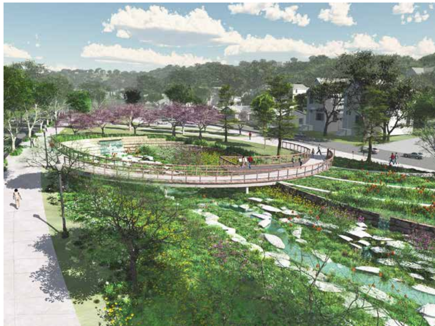
Above: Looking northwest from Westwood Avenue toward Queen City Avenue. This image depicts the daylighting of stormwater into the proposed urban waterway (valley conveyance system). The proposed urban waterway will contain water quality features (limestone rock) and a well-vegetated riparian edge. Rain gardens will help to intercept storm water from Queen City Avenue and direct it to the waterway. (Conceptual Rendering by Human Nature, Inc., of Cincinnati, Ohio)
